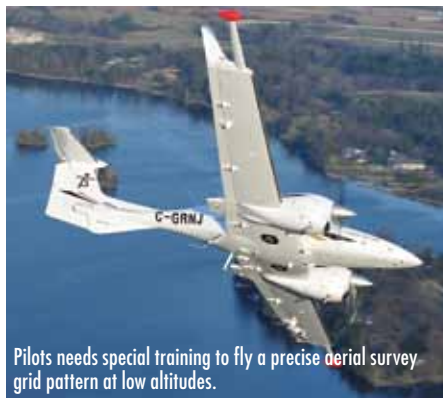
The DA42's long wingspan is good for the magnetometers – the further apart they are, the better the survey data.
